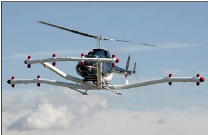
Figure 2 | Helicopter with a magnetometer array
